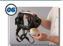
Thread the cartridges or filter assemblies onto the cartridge connectors in the facepiece.
