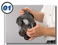
Check the facepiece seal & headstraps to make sure they are in good condition, without any holes or tears. Check the cartridge connectors to make sure they are not cracked and are fully inserted into the mask.
