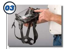
Check the lens to make sure it is not cracked or shows signs of crazing.
